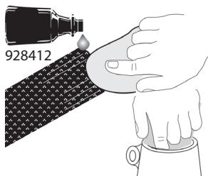
Thoroughly clean end of carbon fiber tube and inside of clamp housing. Use a suitable solvent cleaner such as Acetone (928412). Allow to dry. DO NOT HANDLE CLEANED AREAS.
