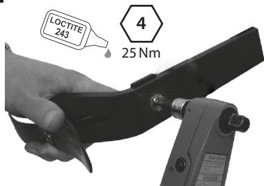
Attach pylon to carrier. Loctite (243) & tighten bolt (25 Nm).
