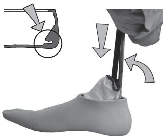
Ensure heel spring is engaged into slot.
