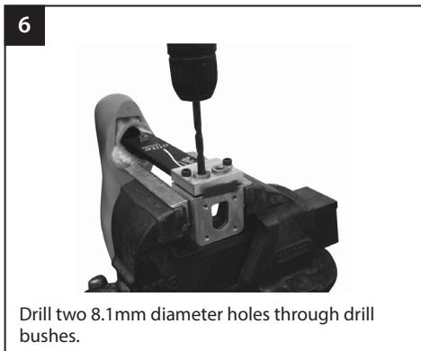
Drill two 8.1mm diameter holes through drill bushes.
