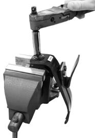
Attach the toe spring to the carrier using Loctite 243 (926012) on the bolts.
