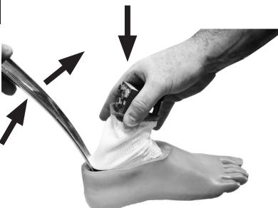
Slide a metal shoe horn between heel spring and back of foot shell opening and lever the spring down into the foot shell.
