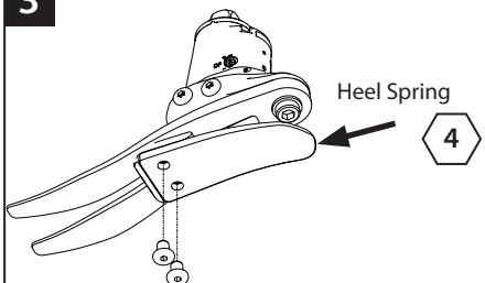
Remove heel spring and screws.
