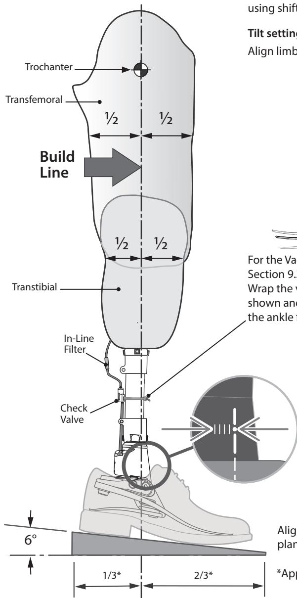
Align transfemoral devices according to fitting instructions supplied with the knee.
