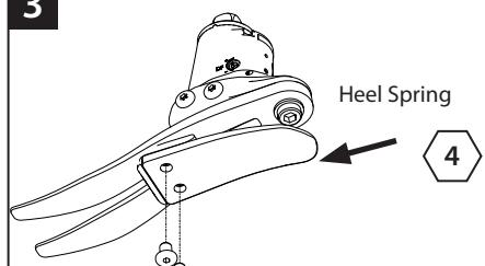
Remove heel spring and screws.
