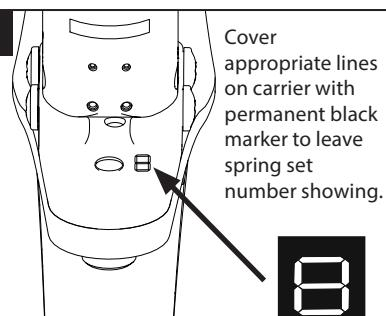
Cover appropriate lines on carrier with permanent black marker to leave spring set number showing.
