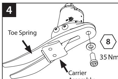
Remove toe spring screw, replace toe. Upon reassembly, use Loctite 243 (926012) and torque to 35 Nm. Ensure toe spring is central to the carrier.
