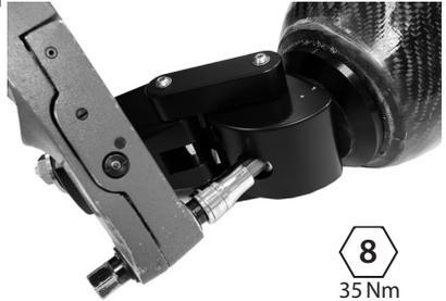
Apply Loctite 243 and torque the proximal alignment bolt to 35 Nm. Use a peg spanner (940060) to prevent the socket plate from rotating.
