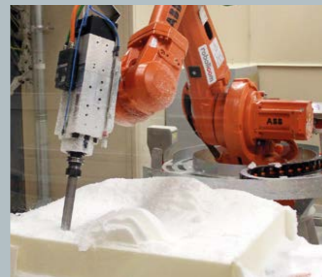
7 Axis robot carved high density HR foam
