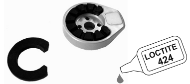
Fig. 2. Medium Buffer Fitted
